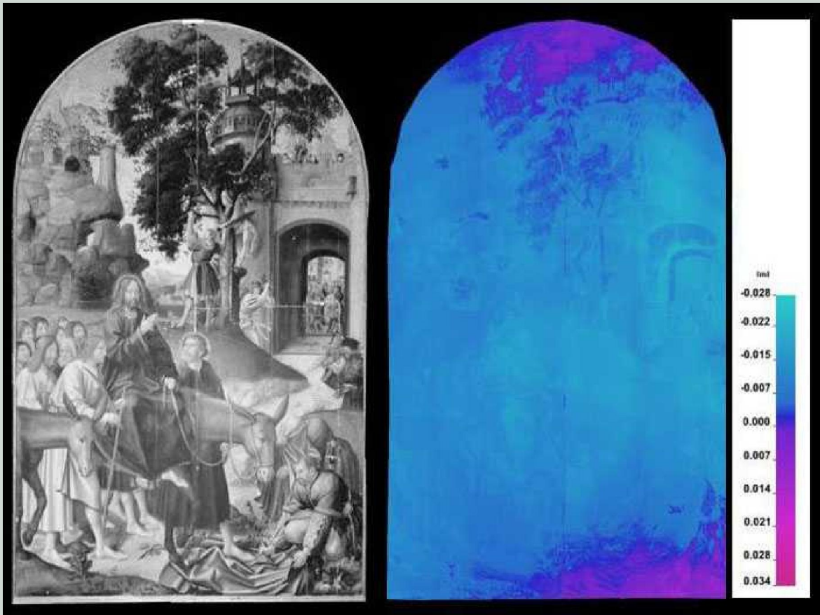
Figure 13. Orthophotography made with laser infrared reflectance and topographic mapping (© Superfície-Geomática, Lda.).
