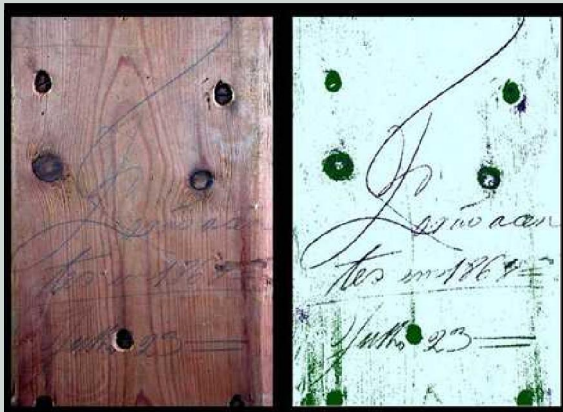
Figure 13. Orthophotography made with laser infrared reflectance and topographic mapping (© Superfície-Geomática, Lda.).
