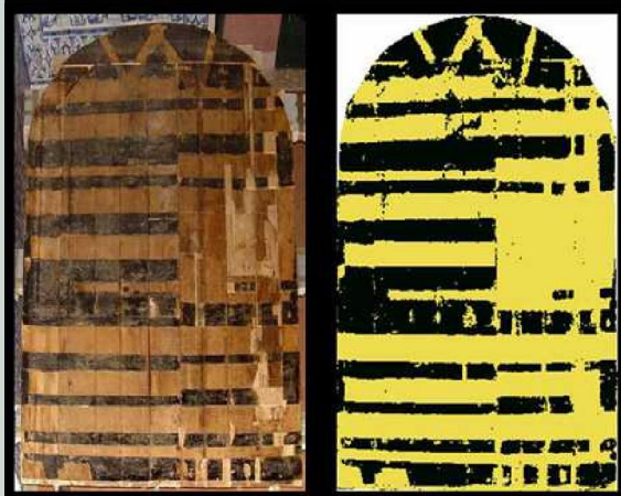
Figure 14. Inscription obtained by supervised classification. Figure 15. Shellac area detection by supervised classification (in black).
